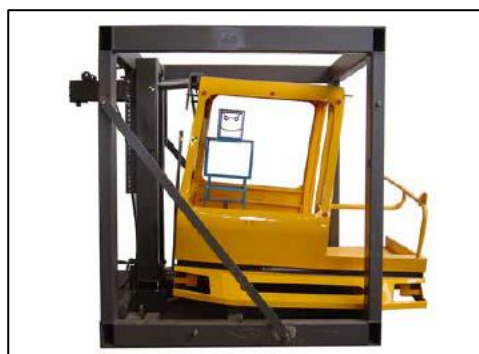
Strong, all-steel cab structure (fully FOPS and ROPS tested) ensures maximum driver protection
