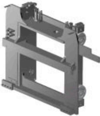
Carriage with passive levelling, standard on DCF80-90 for single stacking
