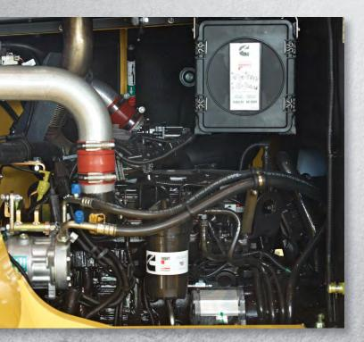
NOTE: A Stage IIIB engine must run on Ultra Low Sulphur Diesel (ULSD) fuel, with a maximum of 15 ppm sulphur content. Diesel fuel with a higher sulphur content than 15 ppm will compromise the emissions performance of the Stage IIIB engine and may result in damage to components. CCC of Stage IIIB engines.
